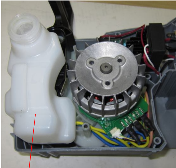
Oil tank assembly
