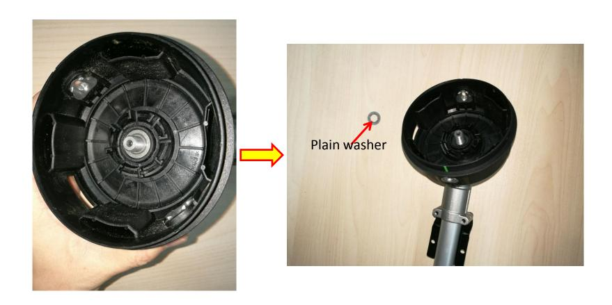
8. Take the upper housing assembly out of the shaft.
