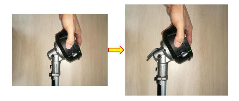
22. Mount the nut onto the shaft and tighten it with multifunction wrench anticlockwise.
