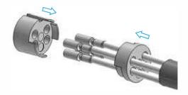
Insert the metal body of the electrical connector at the back of the multicoupling. Insert the cable with all the group assembled on. Allow the alignment of the groove on the cartridge with the pin in the hole of the multiconnection.
