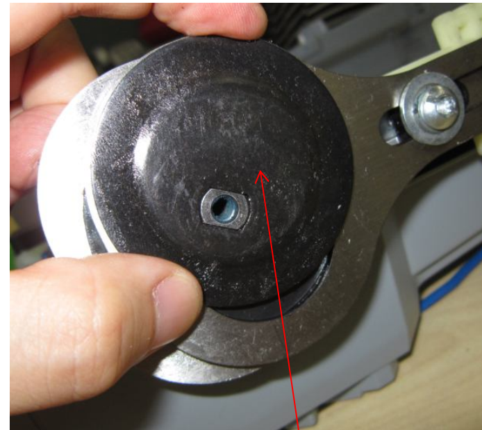
Convexity of the outer washer towards outside
