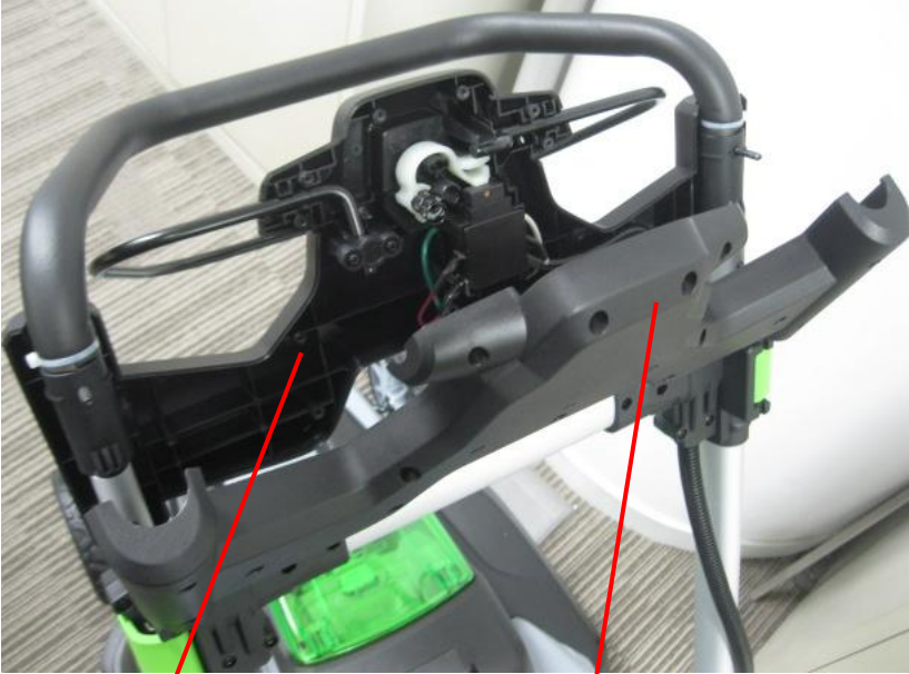
Top switch box cover
