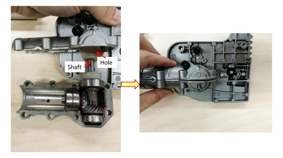
13. Insert the connecting tube assembly into the tube of then gear case assembly and lock them with screws.
