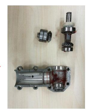
11. Mount the new pinion assembly onto the gear case and then mount the shaft assembly onto
