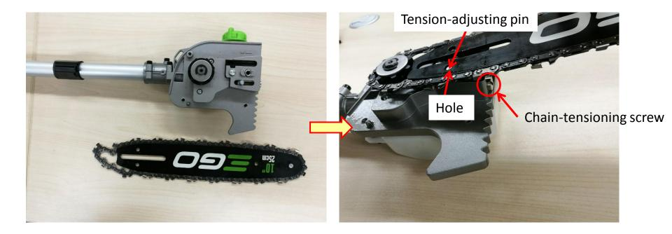
21. Assemble the cover with the gear and chain assembly and tighten them together with screw.
