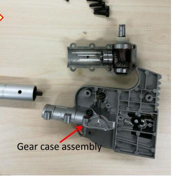
10. Take the pinion assembly and shaft assembly out of the gear case assembly. If the pinion assembly was broken or worn, replace it with a new one.
