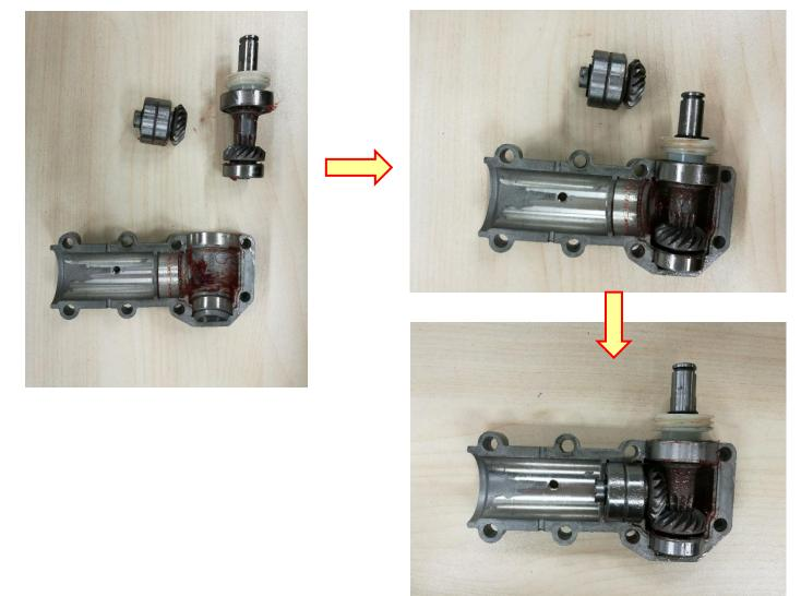
12. Insert the shaft into the hole to assemble the gear case assembly.
