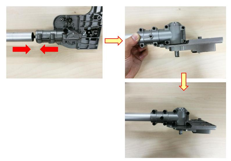
14. Mount the dust cover onto the shaft and assemble the dust cover with the gear case assembly with screws.
