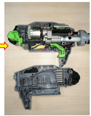
2. Disconnect connector 1 and loosen the screw on the fixed ring.
