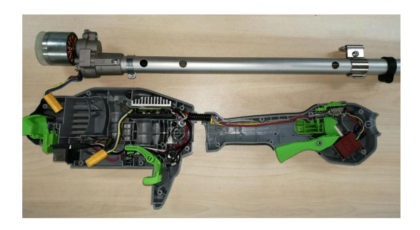
2. Loosen the screw on the gear case assembly to separate the motor and gear case assembly form the shaft assembly.
