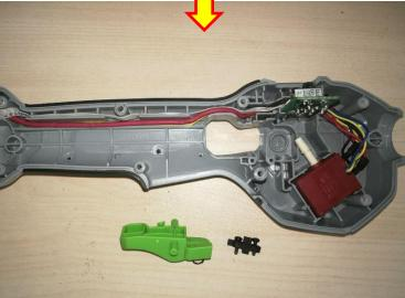
3. Take away the release button, power pack button and lever, if they are broken, replace them with a new one.
