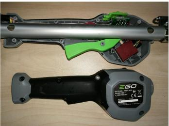
12. Assemble the housing assembly as shown in the "Replace the Motor Assembly" section.
