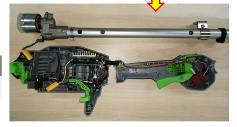
5. Loosen 3 screws to separate the motor from the shaft assembly.
