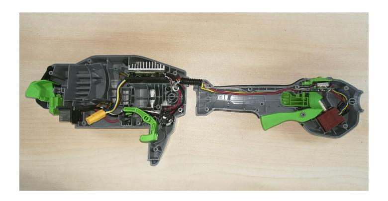
2. Take away the speed change button and switch trigger and then loosen 2 screws on the clamp block to take away the interlock trigger, if they are broken, replace them with a new one.
