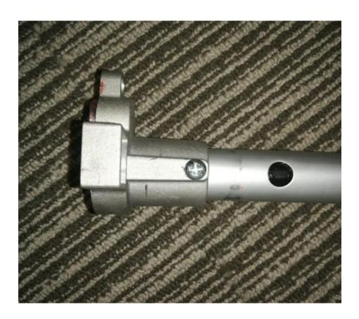
8. Replace the motor with a new one and then assemble the motor with the gear case assembly with screws
