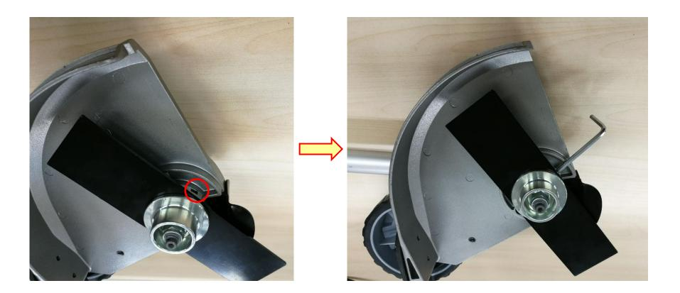
14. Rotate the nut anticlockwise with multifunction wrench to tighten it.
