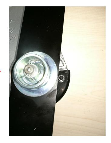
5. Assemble the guide plate with the anti-wear protective guard with screw.
