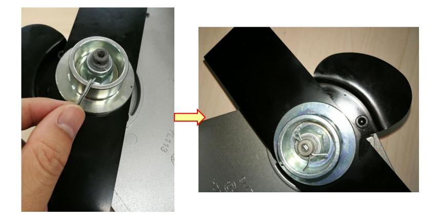
1. Loosen the screw on the guide plate to remove it.
