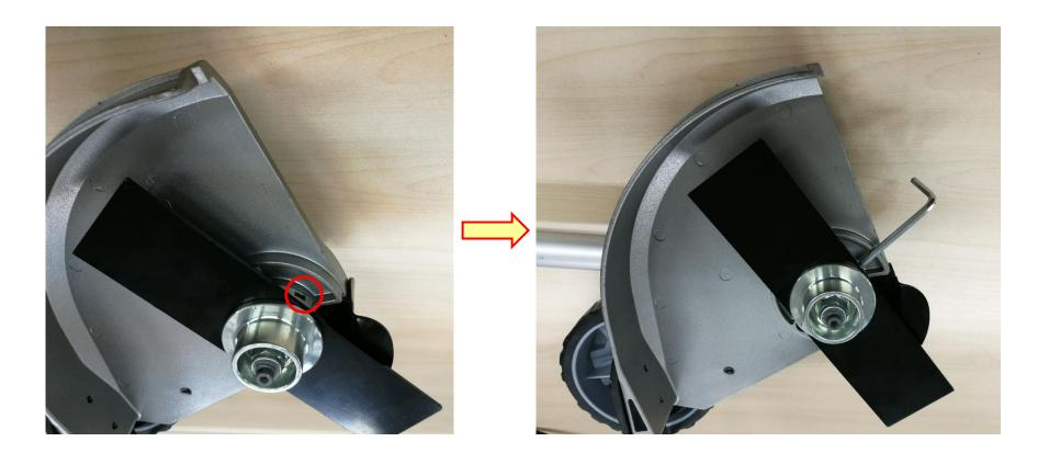
4. Loosen the nut clockwise with the multifunction wrench to remove it.
