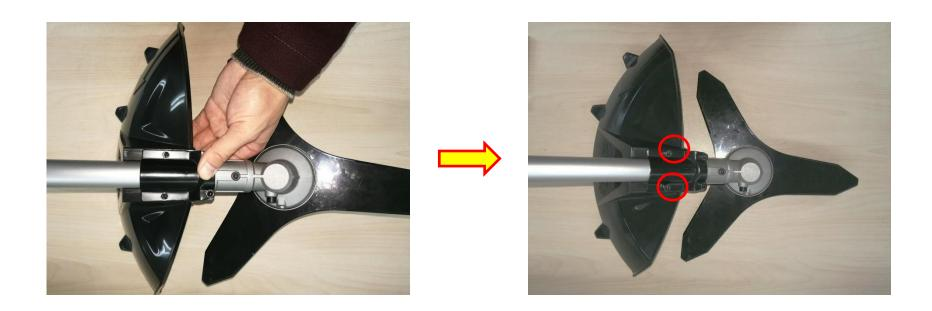
24. Mount the blade onto the blade cover and press the locking bar to assemble them.
