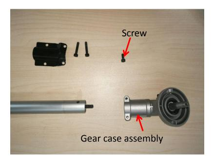
13. Align the hole on the connecting tube with the hole on the gear case and then tighten them together with the screw.
