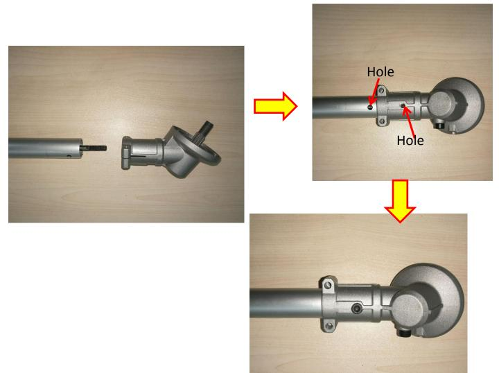
14. Mount the fixing board onto the connecting tube and assemble them with screws.
