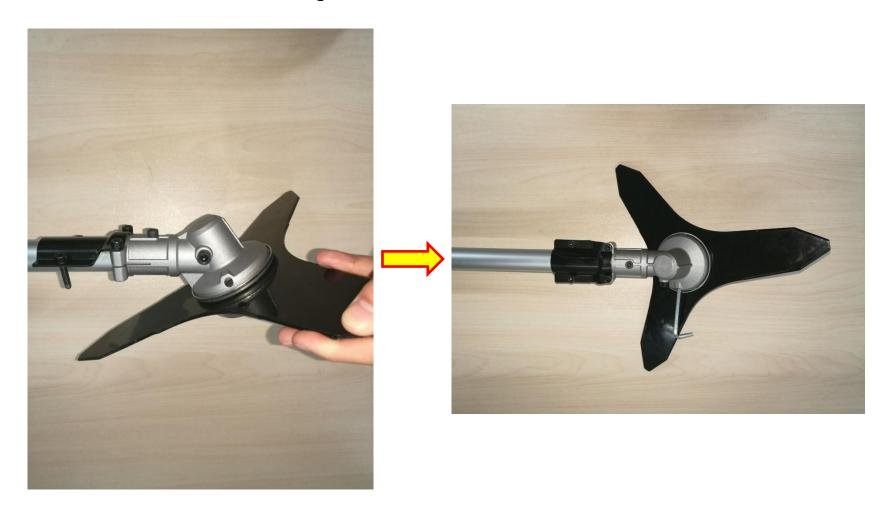
5. Loosen the nut with multifunction wrench clockwise to remove the nut from the shaft.
